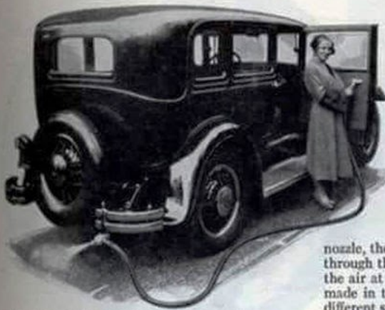
With the car's engine idling, gas from the exhaust creates a vacuum that cleans the cushions
