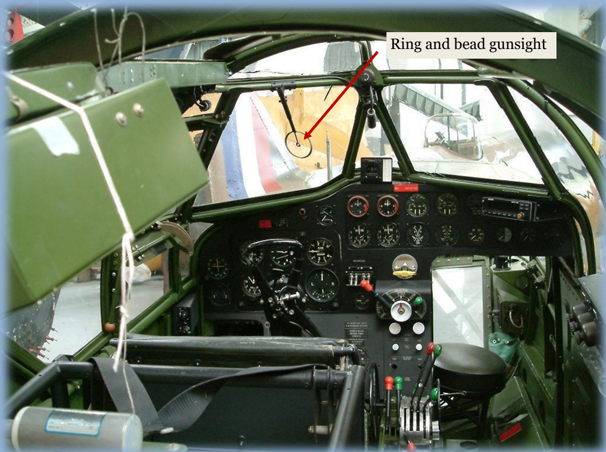
Bolingbroke IV Cockpit (asymmetrical dash due to cut out in nose)
