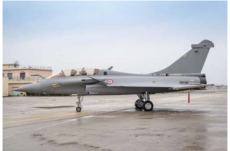
Rafale B359 a two-seat or single-seat, twin engine aircraft with a top speed of 2,222 km/h and a range of 3,700 km.
