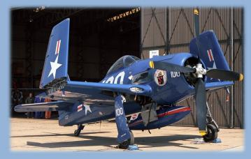
months after the design effort started. The initial flight test demonstrated a 4,800 feet per minute climb rate and a top speed of 424 mph. Compared to the Vought F4U Corsair, the Bearcat was marginally slower but more maneuverable and climbed more quickly.
