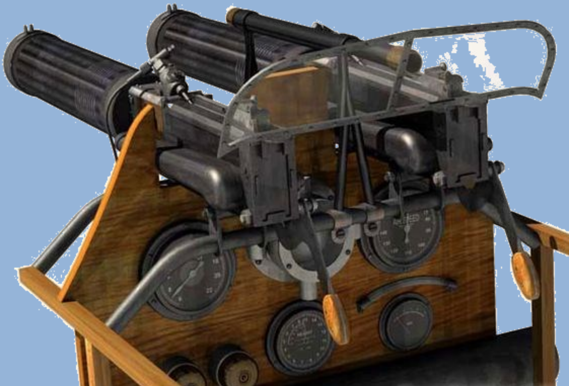
Sopwith Camel Armament: 2 Vickers 7.7mm (.303 in) machine guns with propeller synchronizing mechanism. 4 (25 lb) bombs carried on external racks beneath the fuselage.
