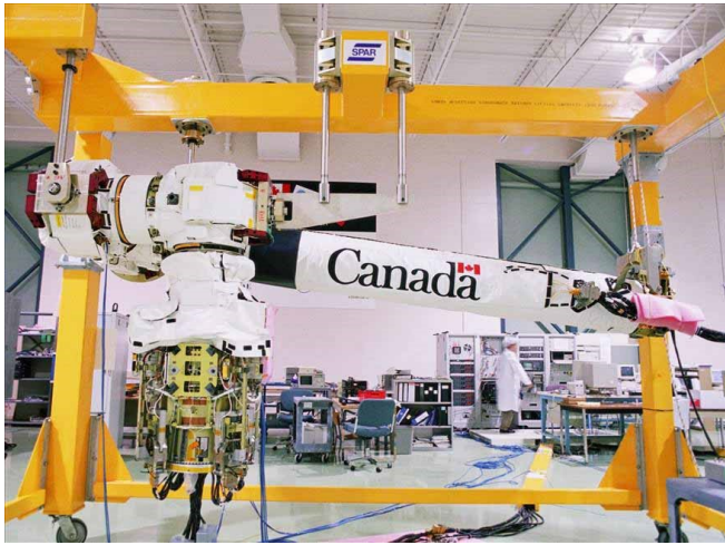
Canadarm2 being assembled and tested at the MacDonald, Dettwiler and Associates Ltd. (MDA) facility in Brampton, Ontario. (Credit: MD Robotics Ltd.)
