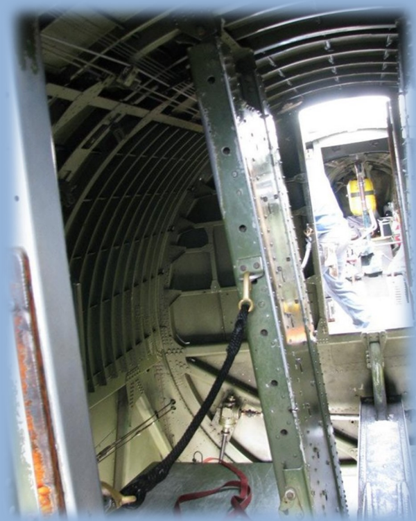
The B-17's rear bomb bay bulkhead with the rectangular access hatch.
